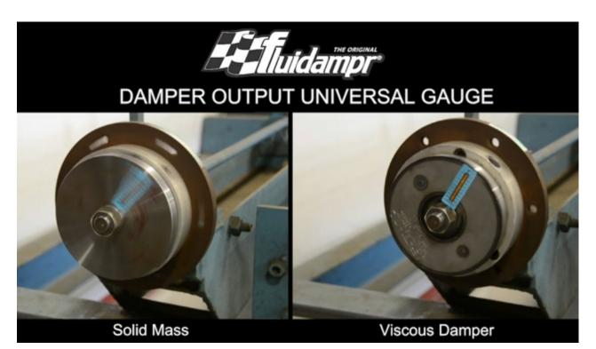
Side-by-side video of a five pound solid mass vs a five pound viscous damper on a validation test rig. When the torsion bar releases it throws each in motion to about 45°. The viscous damper (Right) stops moving in about 15 seconds, while the solid mass keeps moving well over 30 seconds later. **youtu.be/tNLersfbodE**
