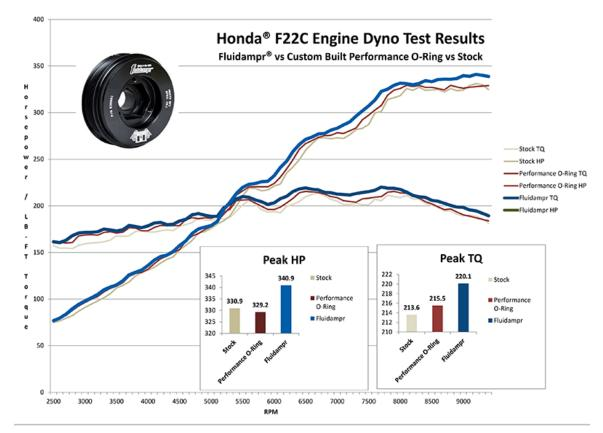
Controlled engine lab testing using a mildly tuned F22C engine on a Superflow water brake engine dynometer at a rate of 1,000rpm per 2 seconds. Only the dampers were changed. Your results may vary.
